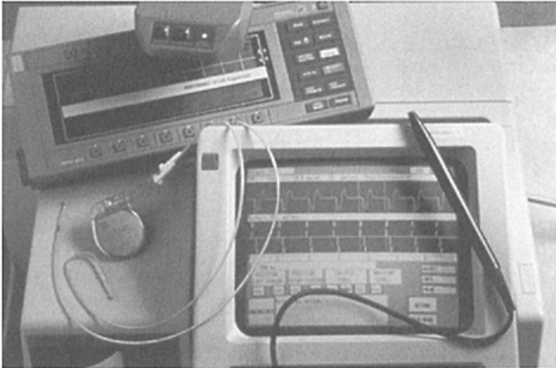
FIGURE 21.1 The pacing systems comprise a programmer, pulse generator, and lead. Two programmers are pictured above; one is portable, and the other is an office-based unit.
