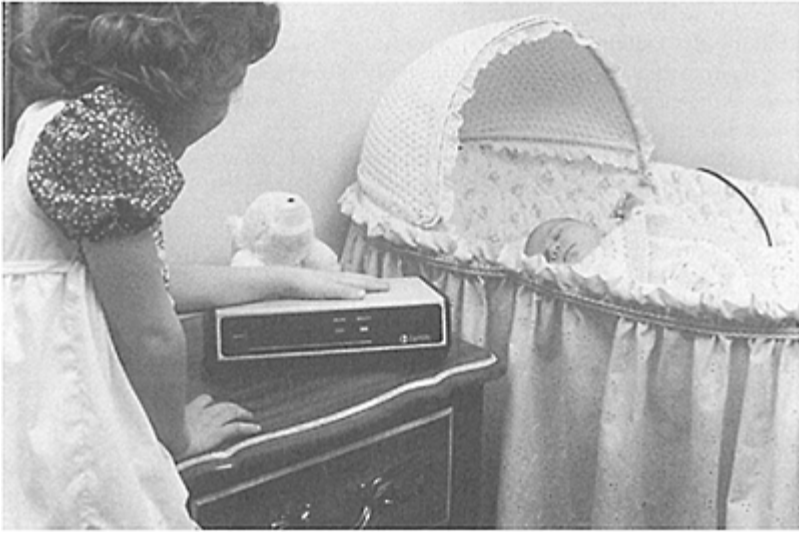
FIGURE 31.1 Infant apnea monitor used in a typical home setting (photo courtesy of EdenTec Corporation).
