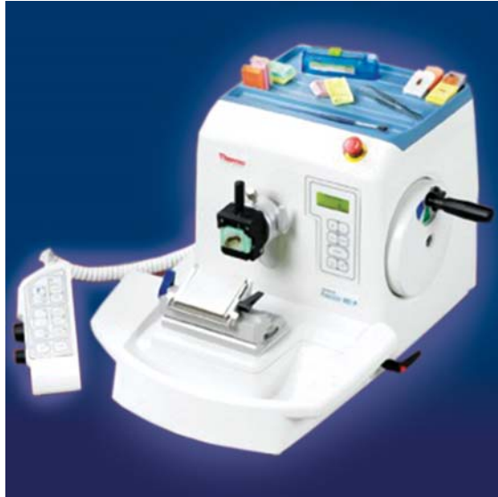
Figure 2.3 ■ Rotary microtome for section cutting by paraffin-embedding technique. (Thermo Shandon, UK). Courtesy: Towa Optics (India) Pvt. Ltd., New Delhi.
