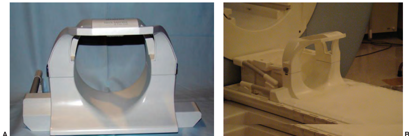
Figure 5.2 Cervical spine coil seen on end (A) and with multisegment attachment (B).
