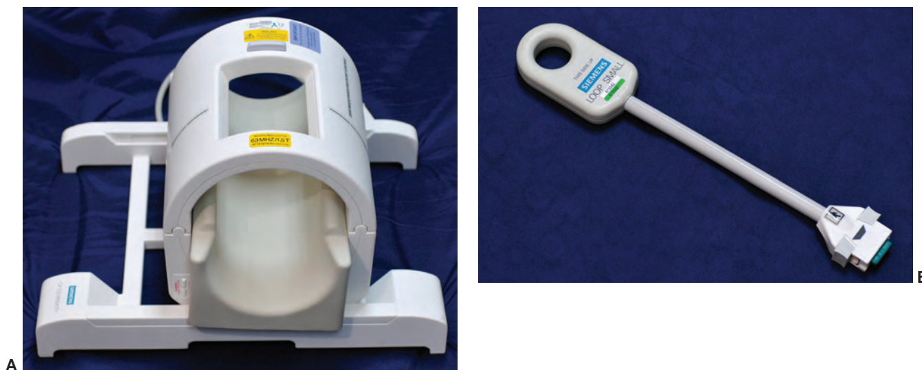
Figure 8.2 Extremity (A) and high detail digital (B) coils used for foot and ankle imaging. (From Berquist TH. Imaging of the Foot and Ankle . 3rd ed. Philadelphia, Lippincott Williams & Wilkins; 2011.)
