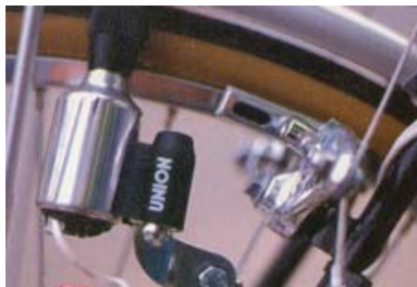
A dynamo converts mechanical energy into electrical energy.
