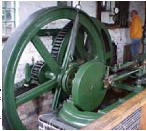
A flywheel stores energy when the supply is in excess and releases energy when energy is in deficit.
