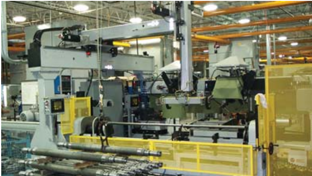
This machine performs pressing operation, welding operation and material handling.
