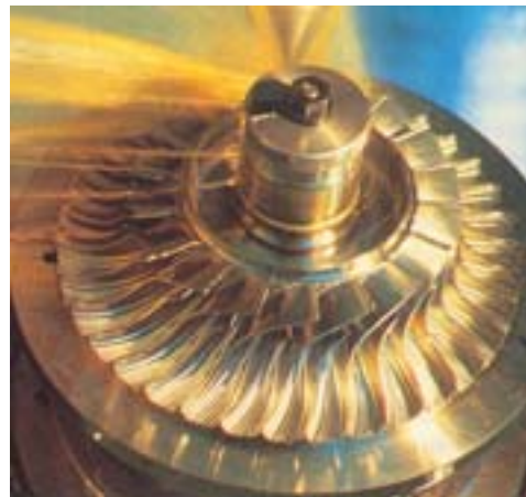
Nowadays steam turbines like this can be produced entirely by computer-controlled machine tools, directly from the engineer's computer.
