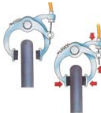
When brakes are on, the pads grip the wheel rim from either side, friction between the pads and the rim converts the cycle's kinetic energy into heat as they reduce its speed.
