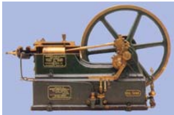
The above picture shows the reciprocating parts of a 19th century oil engine.
