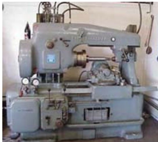
A gear-cutting machine is used to cut gears.
