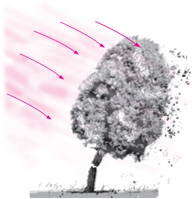
FIGURE 11-4 High winds knock down trees, power lines, and even people as a result of the drag force.
