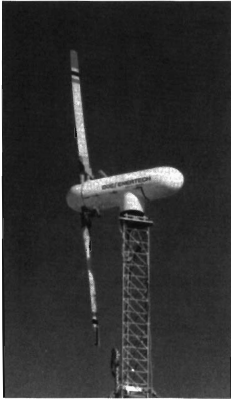
(a) Horizontal-axis wind turbine
