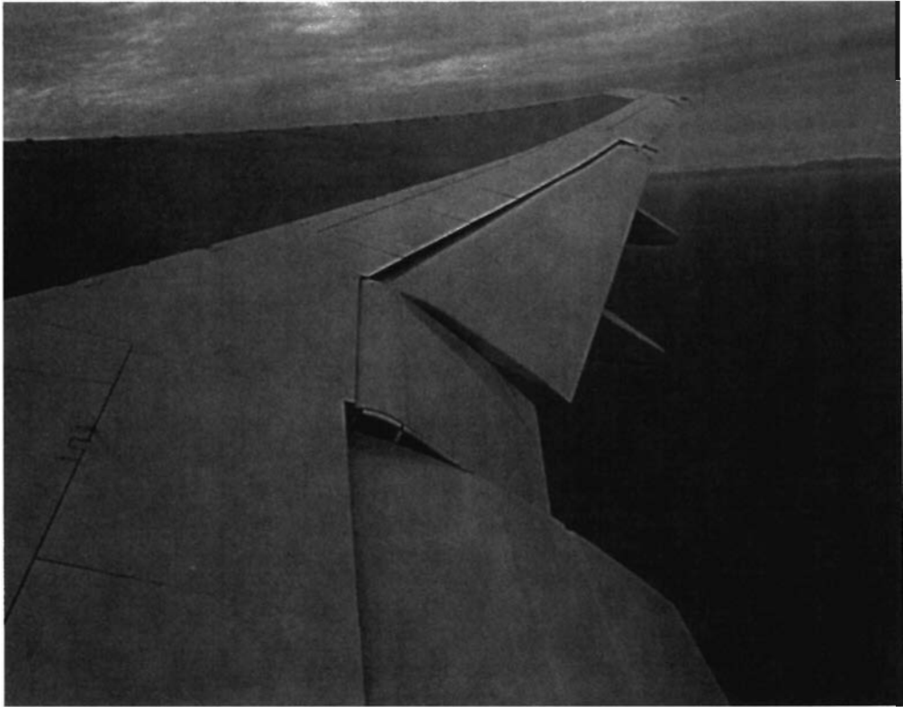
Fig. 9.24(b) Application of high-lift boundary-layer control devices to reduce takeoff speed of a jet transport aircraft. This is another view of the Boeing 777 wing. In the takeoff configuration, large slotted trailing-edge flaps deflect to increase the lift coefficient. The low-speed aileron near the wingtip also deflects to improve span loading during takeoff. This view also shows the single-slotted outboard flap, the high-speed aileron, and nearest the fuselage, the double-slotted inboard flap. (Photograph courtesy of Boeing Airplane Company.)
