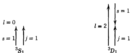
Figure 17-1 Vector addition diagrams showing the spin, orbital, and total angular momentum quantum numbers s , l , and j in the two component states of the deuteron. In the dominant state, l = 0 . Since j = 1 it is necessary that s = 1 in this state which, in spectroscopic notation, is designated {}^3S_1 . In the less probable state, l = 2 . Since j = 1 , it is also necessary in this state that s = 1 . The state is designated {}^3D_1 .
