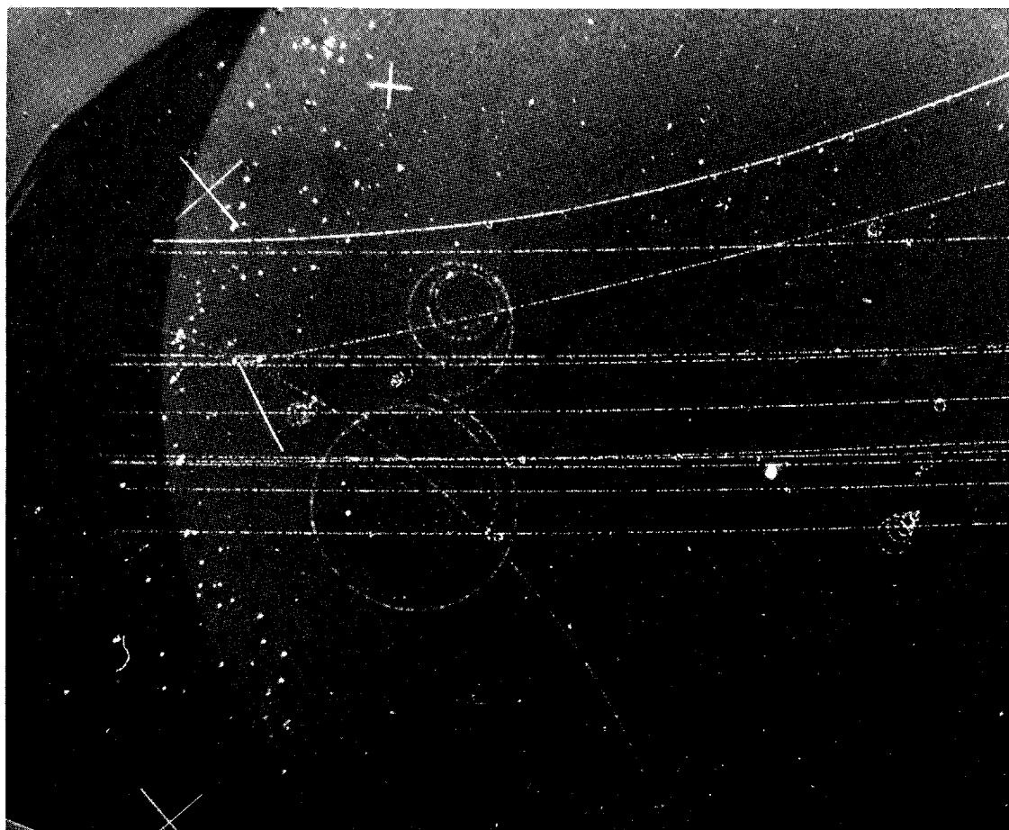
Figure 2-13 Electron pair production, as seen in a bubble chamber. The electron and positron tracks are the two spirals meeting at the point where the production took place in the liquid filling of the chamber. The student can determine which of the two spirals belongs to the positron by knowing that the long tracks are primarily positively charged deuterons which are incident from the left. (Courtesy of C. R. Sun, State University of New York at Albany)
