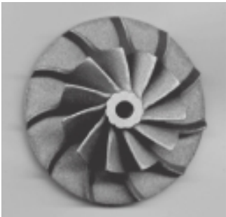
Figure 11.25. Typical geometry of a centrifugal pump impeller. Note how the leading edge of the blade is turned toward the incoming flow direction.
