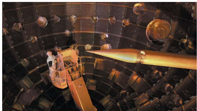
FIGURE 13.18 Workers inside the 10-m-diameter target chamber where 192 laser beams (which enter the chamber through the circular ports) strike the target that is held by the positioning arm at the right.
