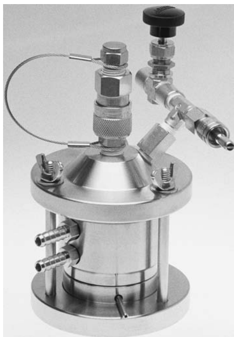
Figure 1 A research scale extrusion device (Lipex TM Extruder) manufactured by Northern Lipids (Vancouver, BC, Canada) has a 10-mL capacity and can be operated over a wide range of temperatures when used in combination with a circulating water bath. The quick-release sample port at the top of the unit allows for the rapid cycling of sample through the filters.
